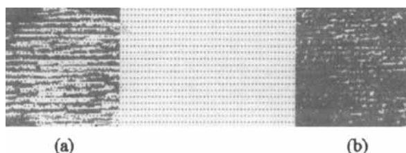
FIGURE 4 Photos of the striped texture in the layer of 4-Chx-2CB. H=5200 Gs (a), H=12300 Gs (b)
